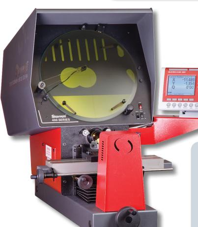
This machine offers a 400mm screen, 250mm x-axis table travel, bayonet fitting lenses and Q-axis angular readout; all to improve capacity and performance.
